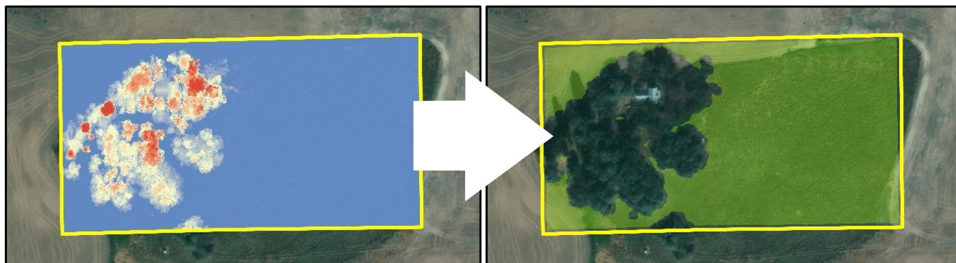
Figure 3. DTM (Digital Terrain Model) is subtracted from DSM (Digital Surface Model) to create a layer which estimates the height of trees and buildings (left) above the ground. By removing areas of tree and building cover, it is possible to demarcate and quantify areas of open space on a parcel, marked in green (right).
