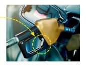
Topping off is not recommended because it may interfere with the proper operation of the vehicle's emission controls. Emission controls are designed to allow for the expansion of gas vapors inside the vapor volume space. The vapor volume space is shown on the diagram inside of this brochure.
