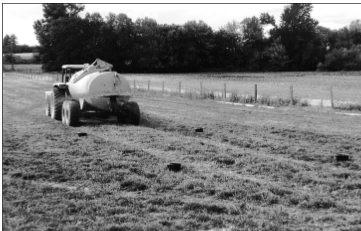
Figure 3. Place several trays, pans, or short buckets in the field to catch liquid applied with one pass.
